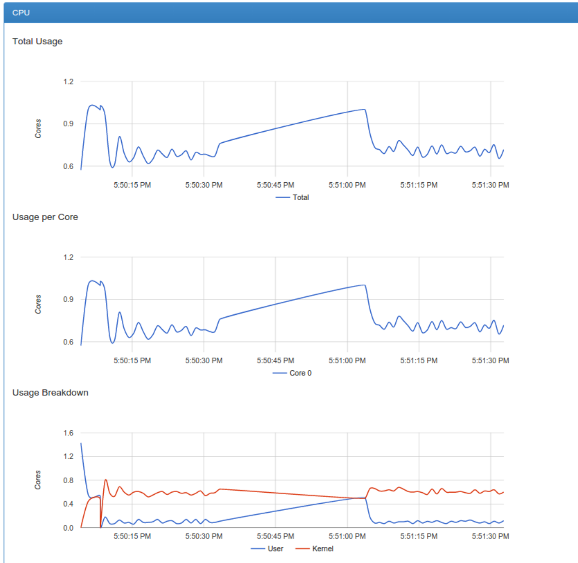
Figure 5: cAdvisor web UI visualizing CPU usage metrics
